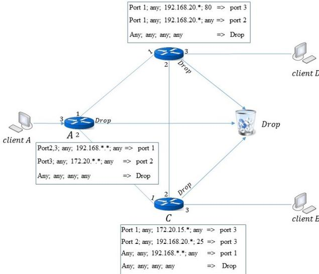
Fig. 2: A Sample network with routing tables
